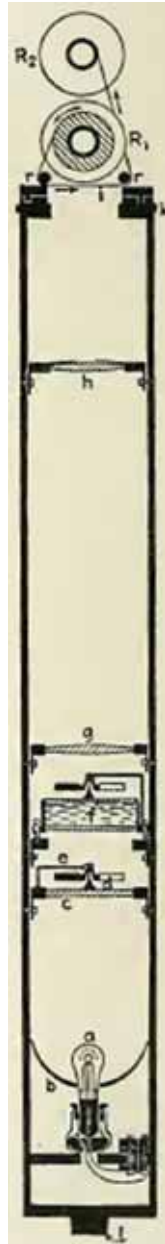
Figure 4: Haussmann's apparatus, showing the film reels (top), lenses, compasses, and light source (bottom)
